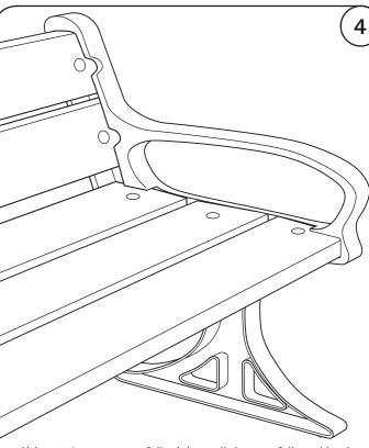
Using a 19mm spanner fully tighten all the nuts followed by the Sleevelocks. See boxes 5 and 6 on the right.
