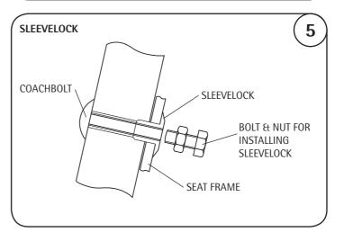
For added security we recommend that the threaded ends of the bolts, on the bottom boards only, are lightly swaged over with a hammer.
