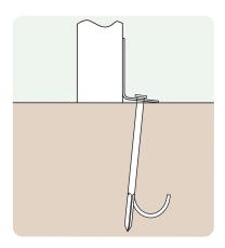
Anchored Soft ground fixing kit for grass.
