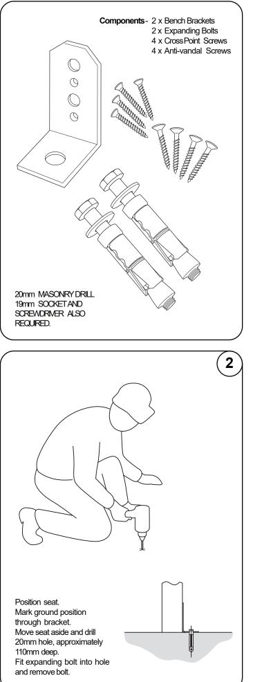
1 Fix 2 bench brackets to the inside of seat legs, diagonally. Mark hole positions through bench brackets, drill 2 pilot holes: 3mm dia x 45mm deep. Fix brackets using either crosspoint or vandal resistant screws. ٠ ▣ 3 Re position seat and fit bolt, but don't fully tighten at this stage. Repeat procedure for the other bolt. When bench is finally positioned, fully tighten both bolts.
