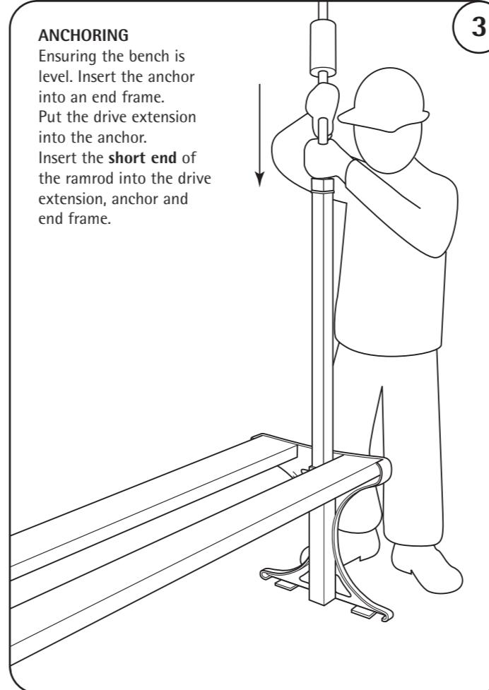
Lift and ram down the ramrod until the anchor collar meets the end frame.
