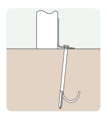
Anchored Soft ground fixing kit for grass.
