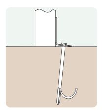
Anchored Soft ground fixing kit for grass.
