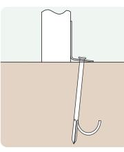
Anchored Soft ground fixing kit for grass.
