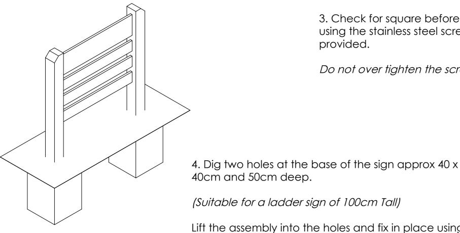
3. Check for square before fixing using the stainless steel screws provided.
