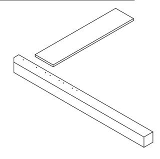
1. Lay a post on the ground with the screw holes facing upwards. (This is the back of the sign)
