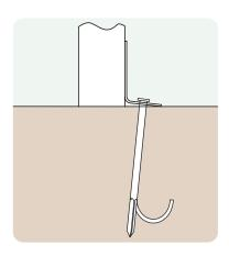
Anchored Soft ground fixing kit for grass.
