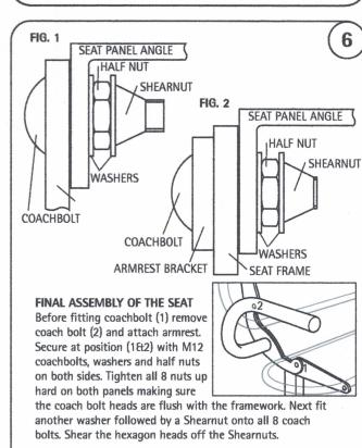
Caution: Shearing of the nuts can usually be sensed but we advise the wearing of gloves during tightening of nuts to
