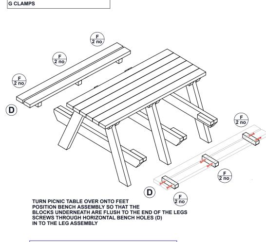
IMPORTANT - USING THE REMAINING 70MM SCREWS THROUGH VERTICAL HOLES AS SHOWN ON PAGE 1 OF 2
