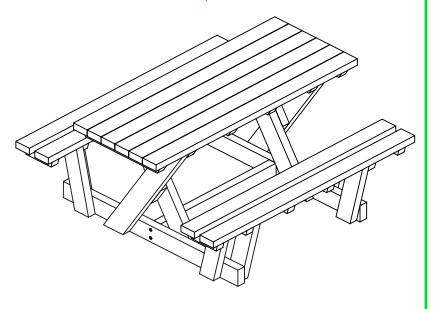
LOWER THE PRE-ASSEMBLED SEAT ONTO THE FRAME AND ALIGN THE HOLES OF THE SEAT TIES WITH THE HOLES ON THE SEAT SUPPORTS
