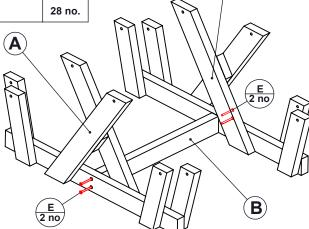
**BEGIN ASSEMBLY WITH THE 2 FRAMES AND** FOOT BRACE SET OUT ON A LEVEL SURFACE
