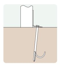
Anchored Soft ground fixing kit for grass.
