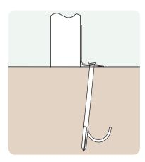
Anchored Soft ground fixing kit for grass.
